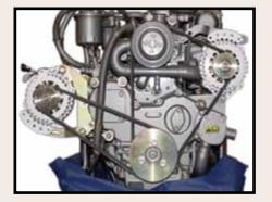
Please note: when using the Centerfielder II in any twin engine application, it is essential that it is used in conjunction with Max Charge MC-614 or MC-624 regulators only. DO NOT use MC-614 regulators with older Centerfielder units.
