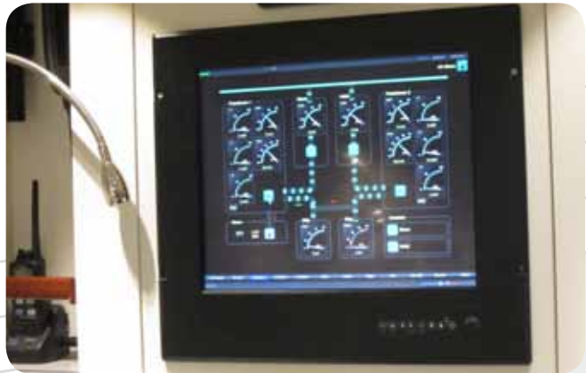
PLC based power management and monitoring for Hybrid systems
