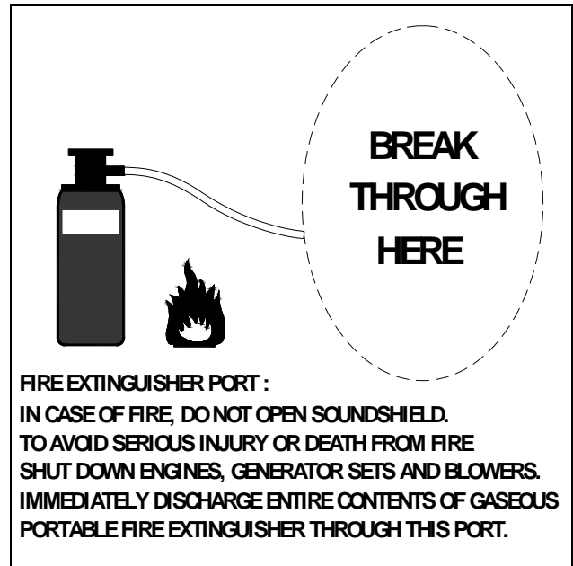
Fig. 3: Fire extinguisher port.
