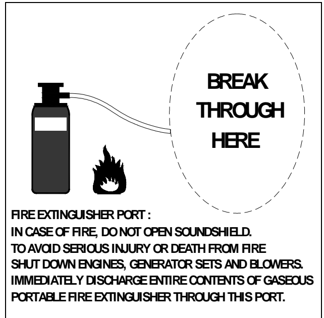
Fig. 2: Fire extinguisher port.
