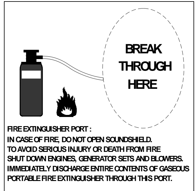
Fig. 2: Fire extinguisher port.
