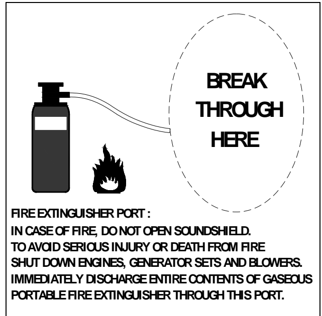
Fig. 2: Fire extinguisher port.
