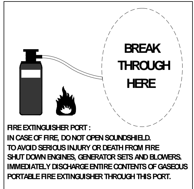
Fig. 2: Fire extinguisher port.
