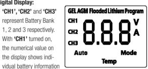
like battery voltage in 'V' or charging current in 'A'. 'CH2' and 'CH3' will always turn on together, the numerical value on the display shows the total charging current in 'A'
