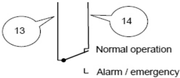
Fig. 20: Connection for emergency stop / fire alarm switch
