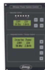
PSCP Power System Control Panel, include Ah counting for servicebattery
