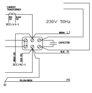
Figure 34: AC wiring diagram
