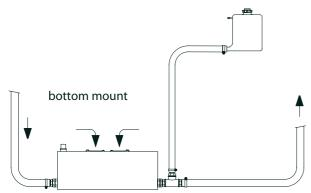
Figure 15. Outgoing connection connected to the expansion tank
