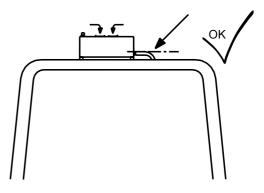
Figure 11: Air traps should be avoided
