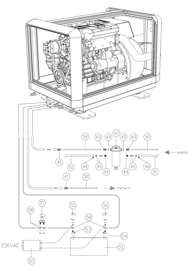
Included are all fittings to fit copper pipes 8 mm outer diameter or rubber fuel hoses 8 mm inner diameter, or both *Figure 29: Installation materials battery and fuel kit*
