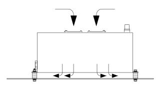
Figure 17. Radiator on rubber mountings
