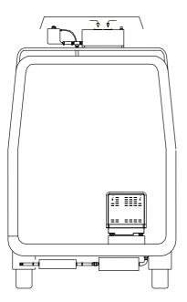
Figure 2: Typical vehicle application radiator top mounted
