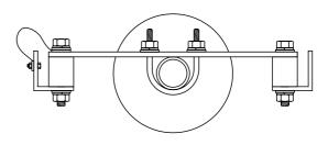
Figure 24. Mounting bracket in rubber with safe guard
