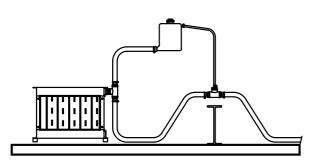
Figure 12: Ventilating an air trap
