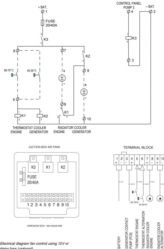
Figure 37: Electrical diagram fan control using 12V or 24V DC radiator fans (optional)
