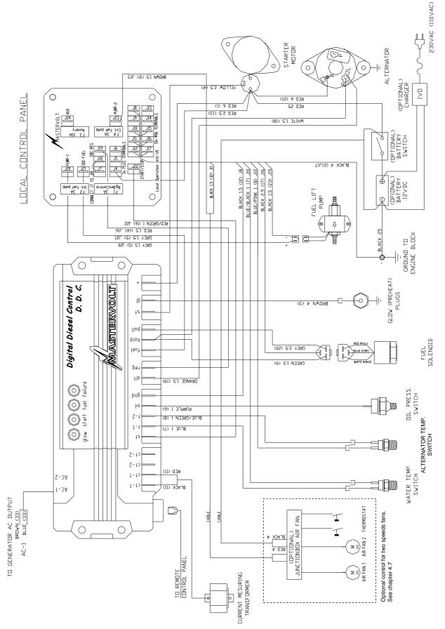
Figure 32: Layout generator control with 12VDC radiator fan
