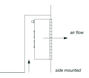
Figure 20: Side mounted radiator
