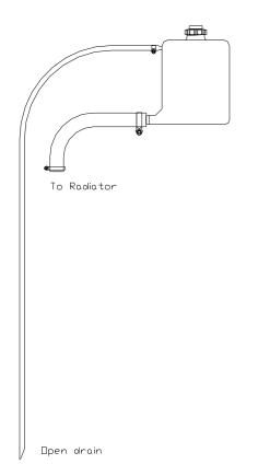
Figure 13. Alternator cooling system: open expansion tank with overflow pillar.
