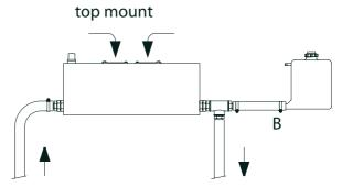
Figure 16: Low profile radiator assembly on the roof
