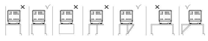
Figure 5: Mounting of the Whisper generating set.
