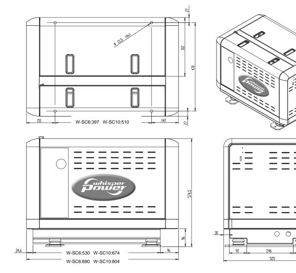
Figure 40: Outer dimensions (mm) W-SC 6 and 10
