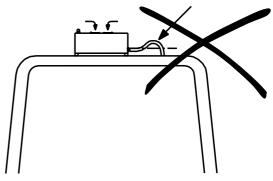
Piping should not be fitted above the radiator!
