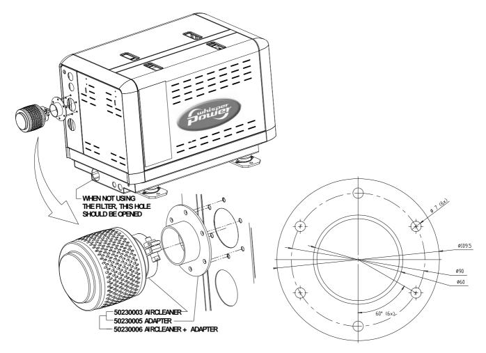
Figure 6: Mounting of the air strainer element
