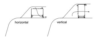
Figure 21: Two examples of top mount radiators
