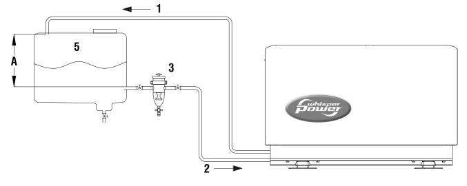
Figure 8: Fuel supply (fuel tank is above the generating set)
