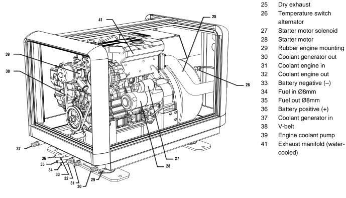
Fig. 5: Rear view main components W-SC 6 and SC10
