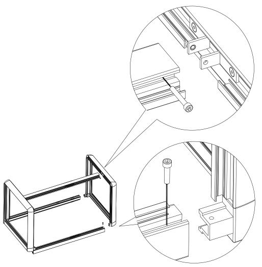
Figure 30: exploded view sound shield W-SC 6 /SC 10
