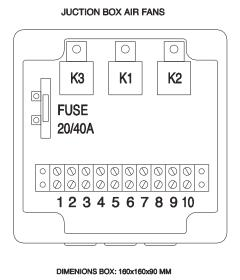
Fig. 16: Electrical diagram fan control using 12V or 24V DC radiator fans (optional)
