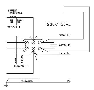
Fig. 13: Electrical diagram 230V
