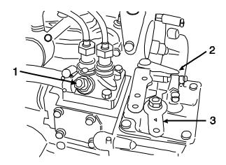
Fig. 19: Bleeding fuel lines 1 = Fuel bleeding screw
